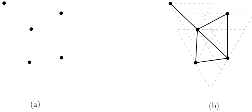
Figure 1.6: A point set P and its G_{\nabla}(P) graph. Edges of G_{\nabla}(P) are shown using thick lines.
