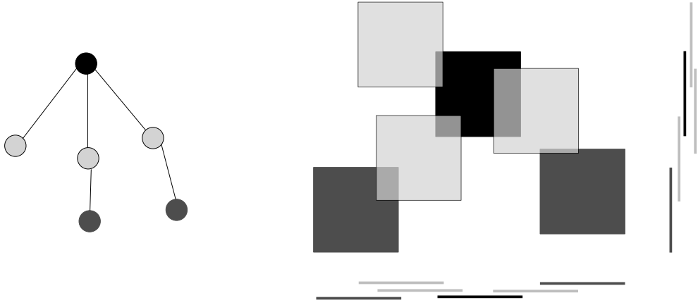
Figure 2.1: A graph and its 2-dimensional cube representation. The projections to X and Y axes give two unit interval graphs.
